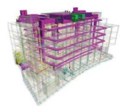
The process produces the **Building Information Model (BIM)**, which encompasses building geometry, spatial relationships, geographic information, and quantities and properties of components. These different views are automatically consistent – in the sense that the objects are all of a consistent size, location, specification – since each object instance is defined only once, just as in reality. Drawing consistency eliminates many errors.
