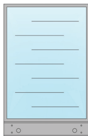
S1 / S2 Silencer Section S1 : 25 dB (A) Loss S2 : 30 dB (A) Loss
